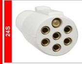
Compatible with all 7-Core Cable(s) listed on page 10 White Common Return 1 2 Black Not assigned 3 Yellow Reversing light Permanent power supply 4 Red 5 Green Sensing device with common return Blue Power supply (controlled by ignition switch) 6 Brown Rear fog light
